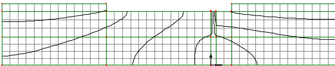
Fig. 3 – Mesh (and contours of potential), with element length set to 1.5m
