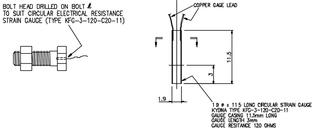
Figure 5 - Strain gauge in situ detail and enlarged detail of gauge
