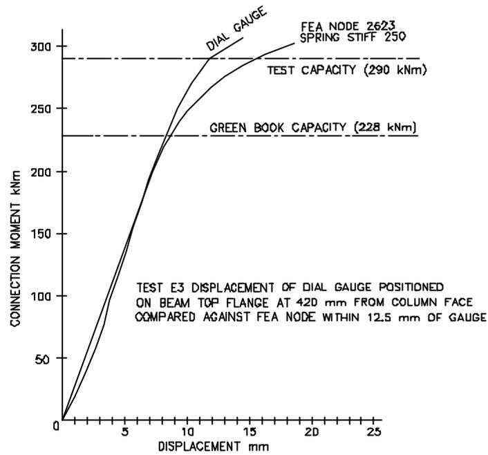
Figure 14 - Test E3 and FEA rotation comparison
