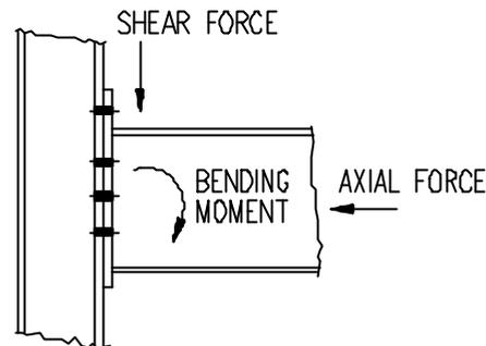
Figure 2 - Connection Loading
