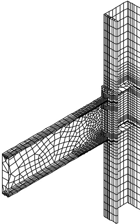
Figure 7 - Mesh Discretisation
