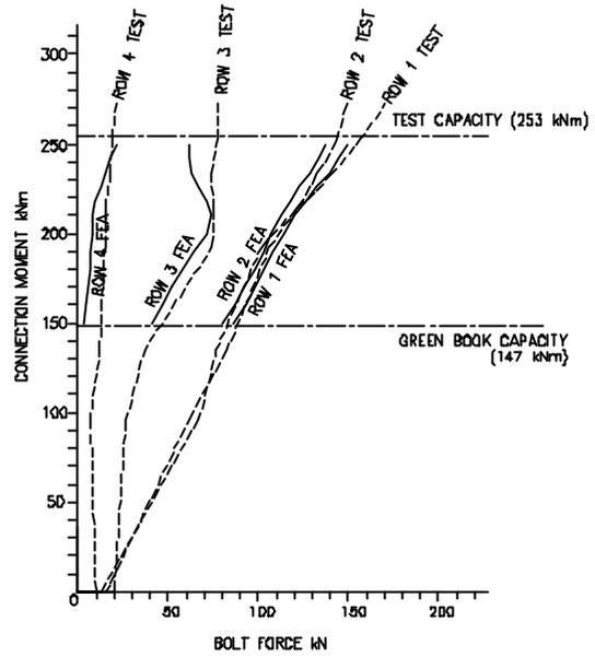
Figure 12 - Test E1 and FEA bolt force comparison    Figure 13 - Test E5 and FEA bolt force comparison
