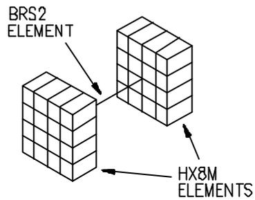
Figure 10 - Enlarged FEA Bolt Arrangement
