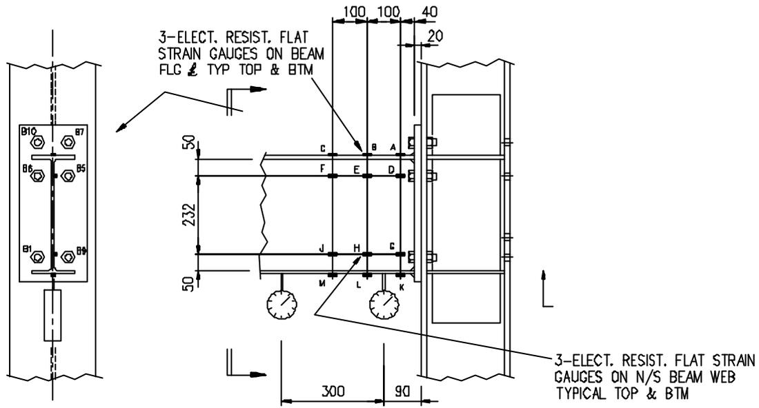
Figure 4 - Strain / Dial gauge locations
