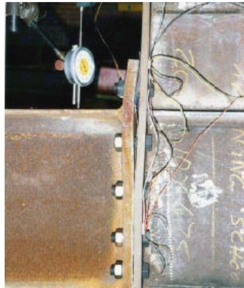
Figure 16 - Test E3 just prior to bolt failure
