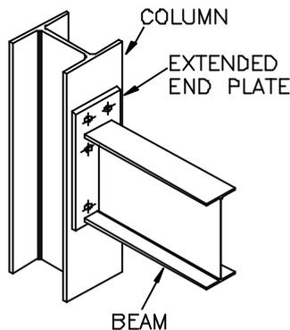
Figure 1 - Extended End Plate Connection
