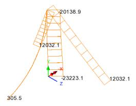
This image shows axial force for the combined effect of the initial stress, the self-weight and the wind loading on the mast.
