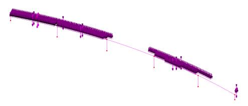
After further inspection (by selecting the line of each span and looking at the filtered results in the onerous results table) it can be seen that the most onerous results for hogging are actually obtained for span 3 at pier 2 (Point 4).
