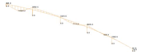
The preceding diagram shows the worst-case sagging moment, My, for span 5, due to characteristic LM1 loading.
