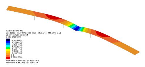
The contours can be simplified to indicate which areas of the structure, when loaded, will have a positive, or negative influence for the selected influence assignment.
