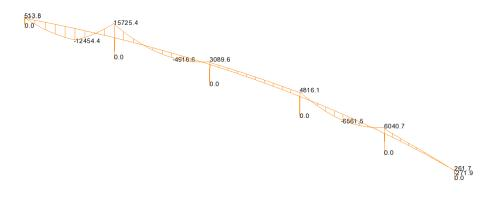
The preceding diagram shows the worst-case hogging moment, My, for span 5, which occurs at pier 4, due to characteristic LM1 loading.
