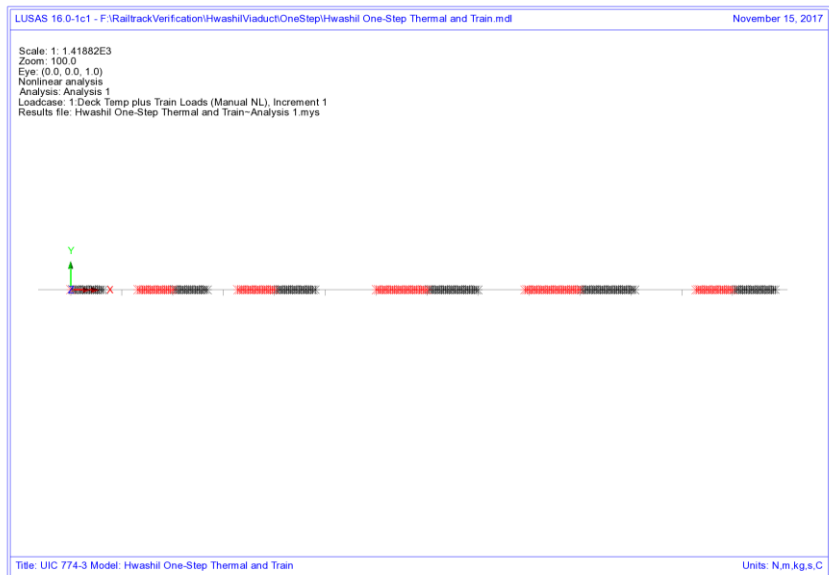
Figure 88: Track/Rail 2 Yield Due To Accelerating Train Loads On Track 2 - Thermal And Rail Applied Concurrently
