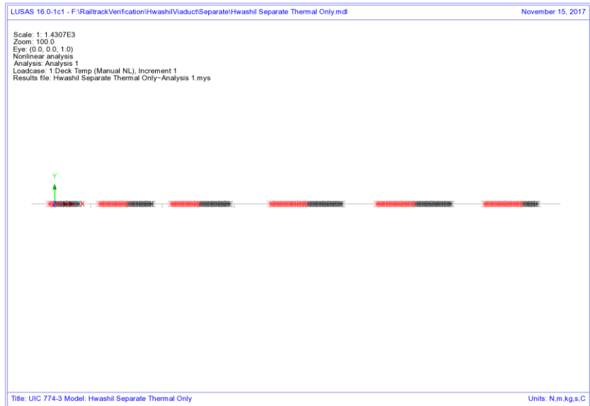
Figure 86: Track/Rail 2 Yield Due To Thermal Load On Track Alone
