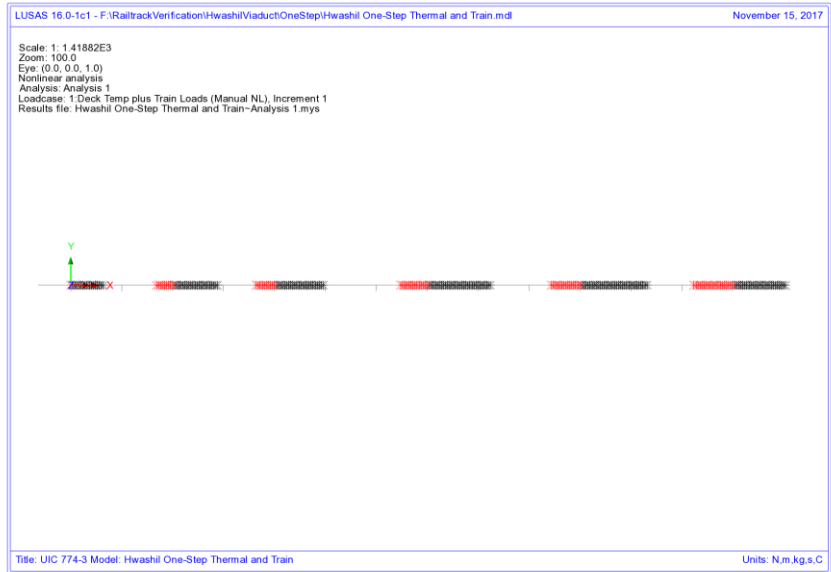
Figure 94: Track/Rail 1 Yield Due To Braking Train Loads On Track 1 - Thermal And Rail Applied Concurrently
