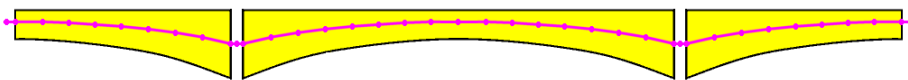
Indicative diagram showing 'Curved' modelling method (where all lines follow the centroid of sections)
