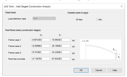
Fig 27 Dialog for Adding Staged Construction Analysis
