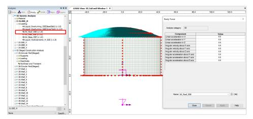
Fig 16 Horizontal Seismic Loading for Roof (SSE)
