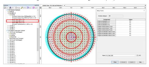
Fig 17 Horizontal Seismic Loading for Wall (SSE)
