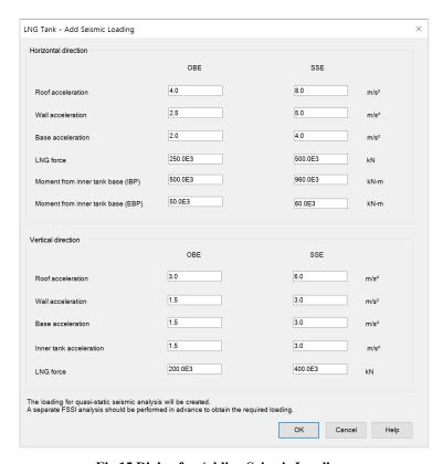
Fig 15 Dialog for Adding Seismic Loadings
