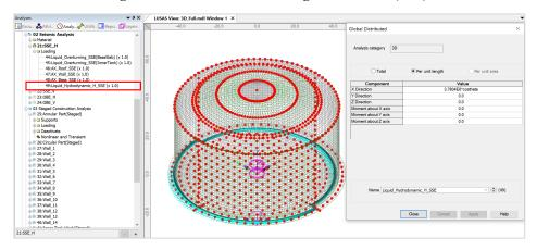
Fig 19 Horizontal Seismic Loading of Liquid Force (SSE)
