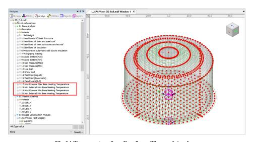
Fig 14 Temperature Loading from Thermal Analyse
