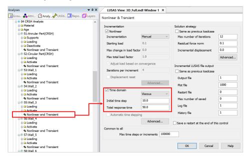
Fig 34 Nonlinear Control for Stage of Wall 2 (Default)
