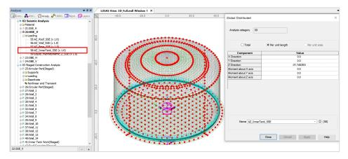
Fig 25 Vertical Seismic Loading for Inner Tank (SSE)
