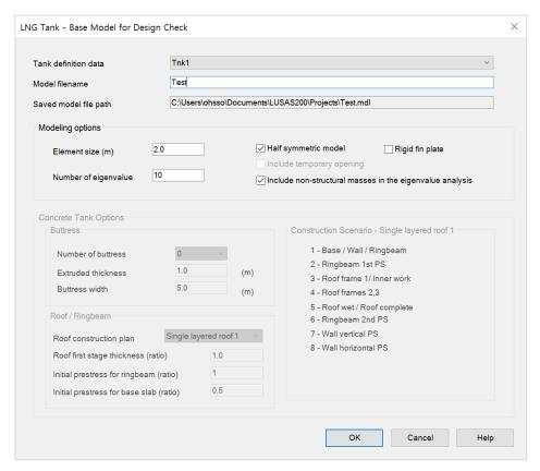
Fig 2 LNG Tank for Base Model for Design Check
