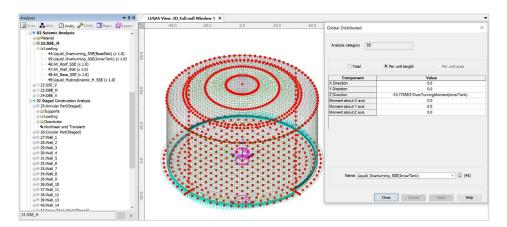
Fig 21 Horizontal Seismic Loading of Overturning Moment from Inner Tank (SSE)
