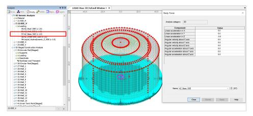
Fig 24 Vertical Seismic Loading for Base Slab (SSE)
