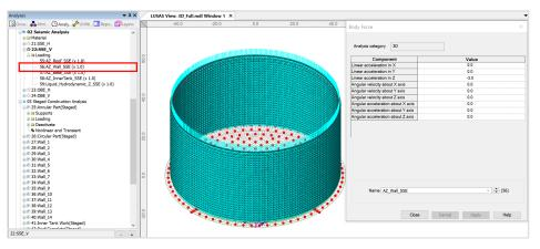
Fig 23 Vertical Seismic Loading for Wall (SSE)
