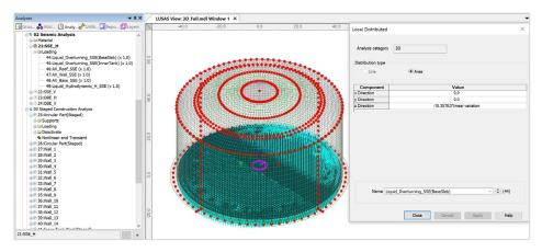
Fig 20 Horizontal Seismic Loading of Overturning Moment from Base Slab (SSE)
