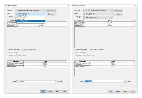
Fig 32 Creep & Shrinkage Material for Base Slab
