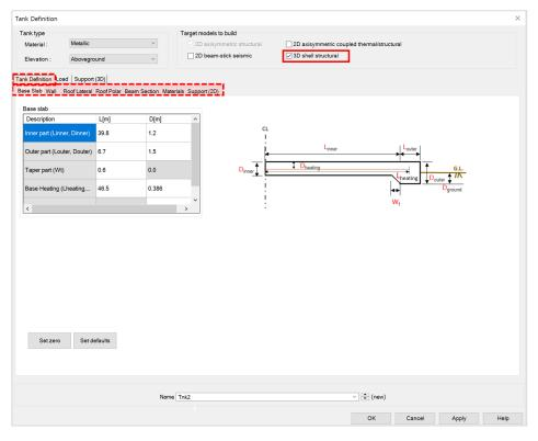
Fig 1 User Input for Tank Dimension and Load
