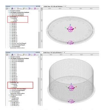
Fig 29 Stage 3 ~ 16 of Staged Construction Analysis
