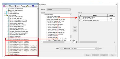
Fig 39 Load Combinations Created in Modeller
