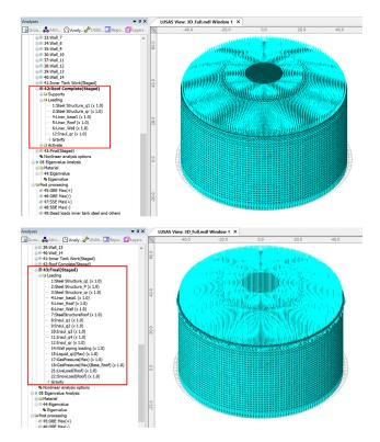
Fig 30 Stage 17 ~ 19 of Staged Construction Analysis
