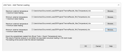
Fig 13 Dialog for Adding Thermal Loading
