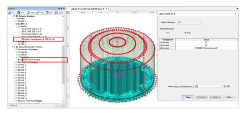
Fig 26 Vertical Seismic Loading for Liquid (Hydrostatic, SSE)
