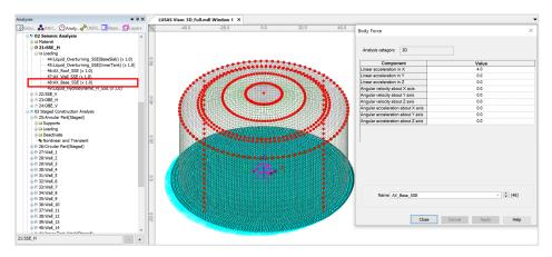
Fig 18 Horizontal Seismic Loading for Base Slab (SSE)
