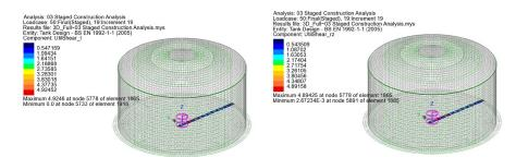
Fig 45 Contour for UtilShear t, UtilShear rv
