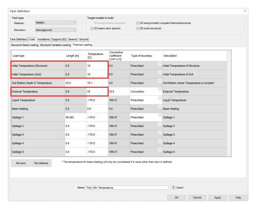
Fig 10 User Input for Min Environmental Temperature
