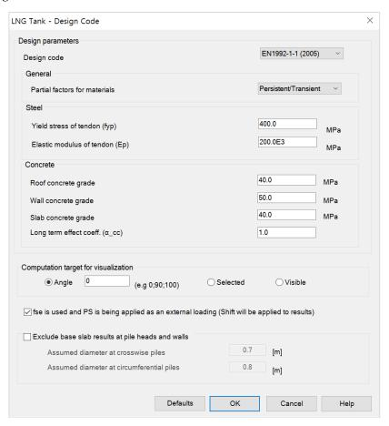
Fig 40 Dialog for Design Parameters
