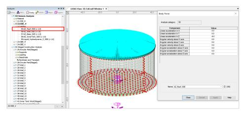
Fig 22 Vertical Seismic Loading for Roof (SSE)
