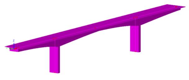
Varying section line attributes assigned to single lines on a model
