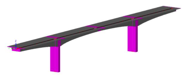
Varying section line attributes (shown selected) assigned to multiple lines on a model with reference to a path
