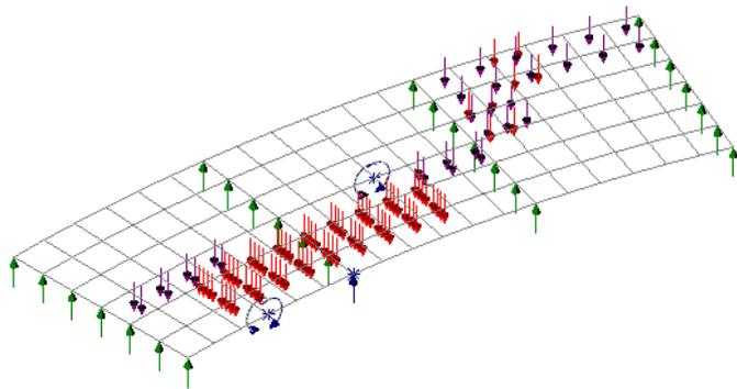
Figure 10. Example of an optimized vehicle loading pattern .
