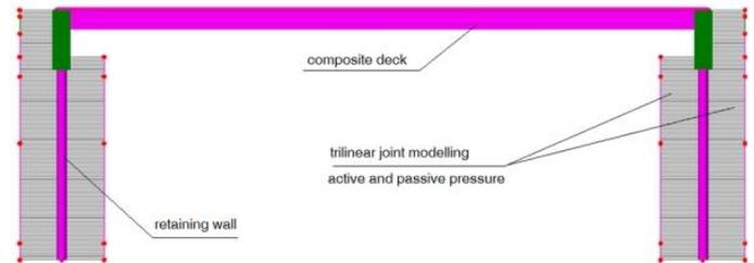
Figure 11. Model of integral bridge designed to EC4.
