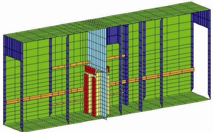
Figure 2. Crosshead modelling on the Midlands Links Viaducts
