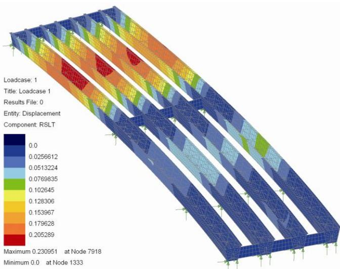
Figure 8. Estero Parkway Flyover: Resultant displacements from deck pour loading.
