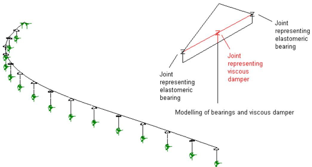
**Fig. 10– Global model of viscous damped road bridge**
