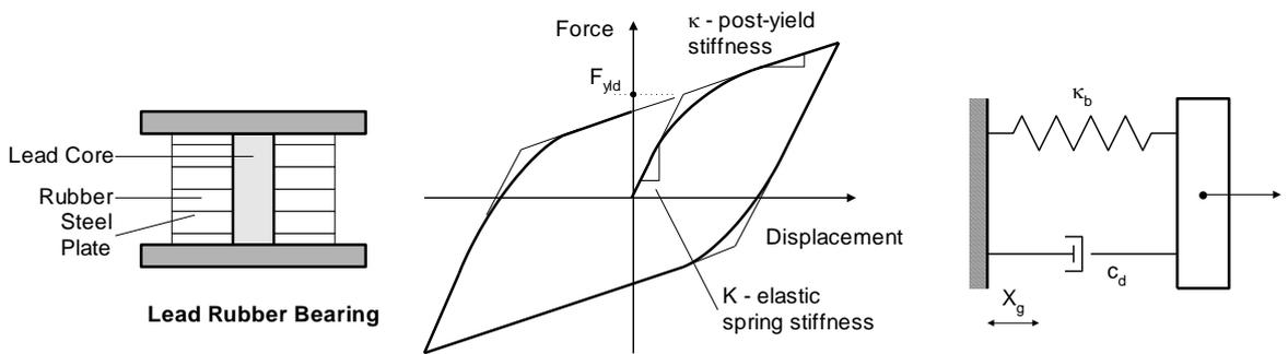
Lead rubber bearing, hysteretic behavior and schematic representation
