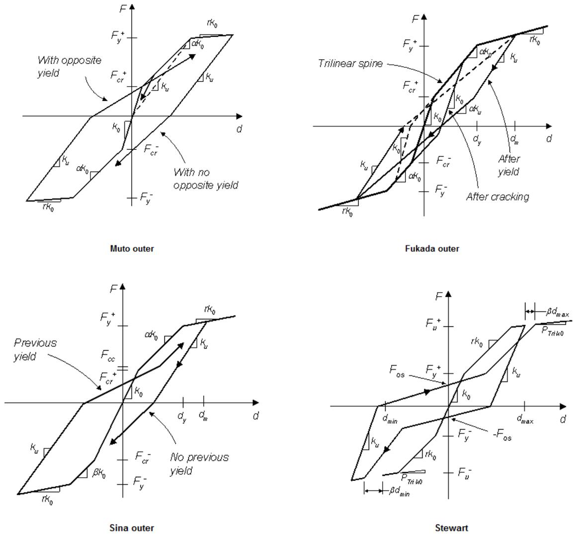
**Fig 3 – Hysteretic joint models to model potential failure in structures**
