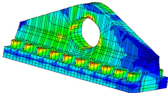
**Fig 14 – Gateshead Milennium bridge bearings**
