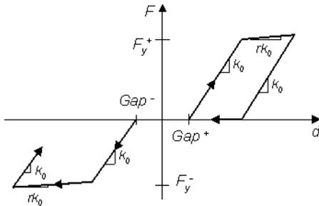
**Kinematic hardening with slackness**
