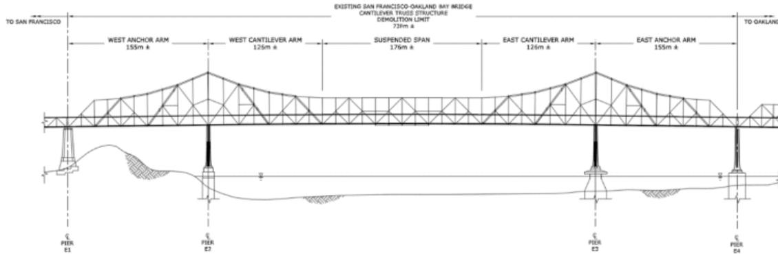
Layout and primary dimensions of the old East Main Span.
