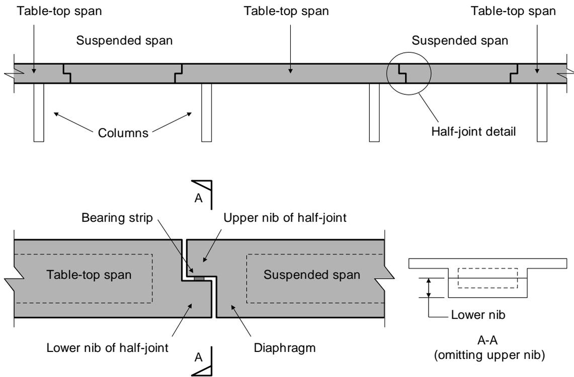
**Fig. 12-Schematic half-joint geometry for Kingston bridge approach ramps**
