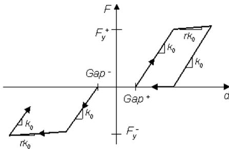
**Kinematic hardening with slackness**
