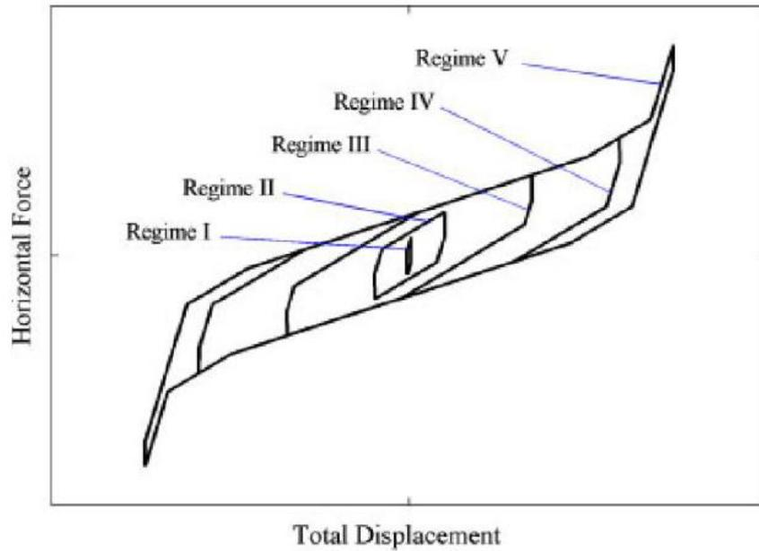
Triple friction pendulum bearing
