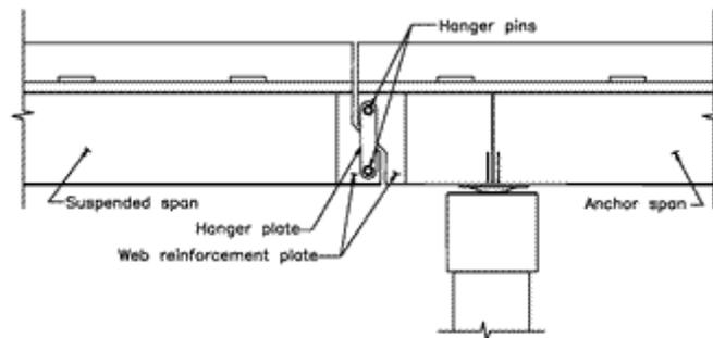
Typical pin and hanger joint
