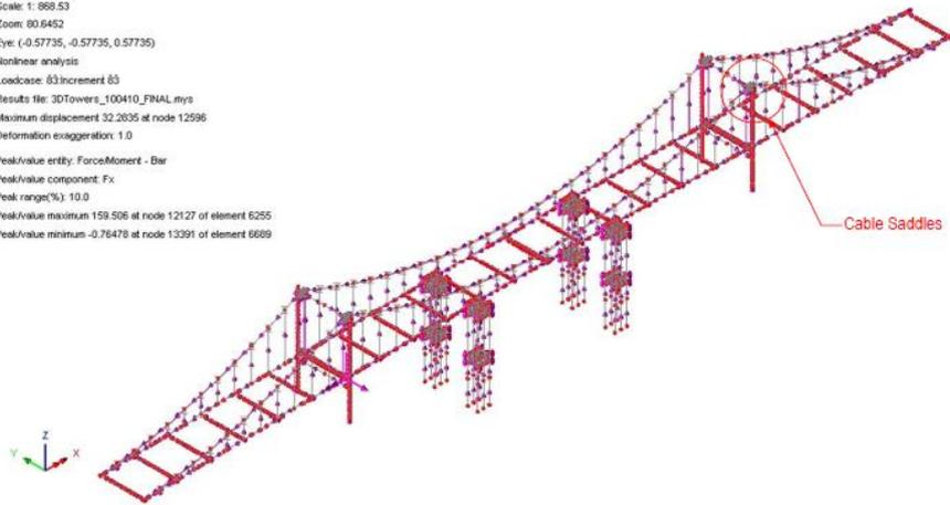
Analysis Model – Included original construction stages to establish existing stresses
