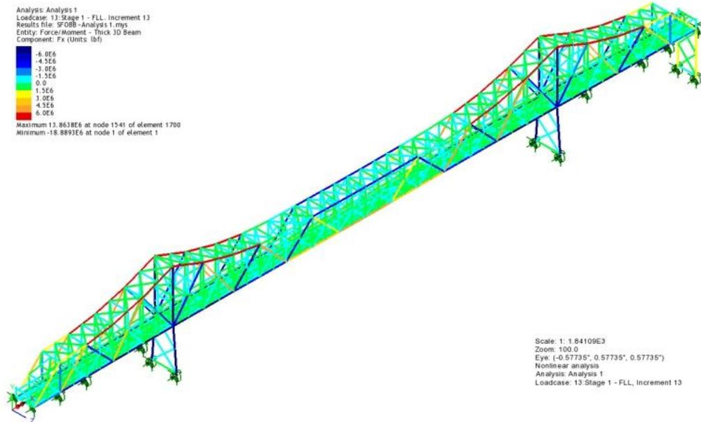
The stringer support at select floorbeams is modeled to accurately account for the slotted-hole longitudinal expansion connection with a "spring stiffness only" joint material.
