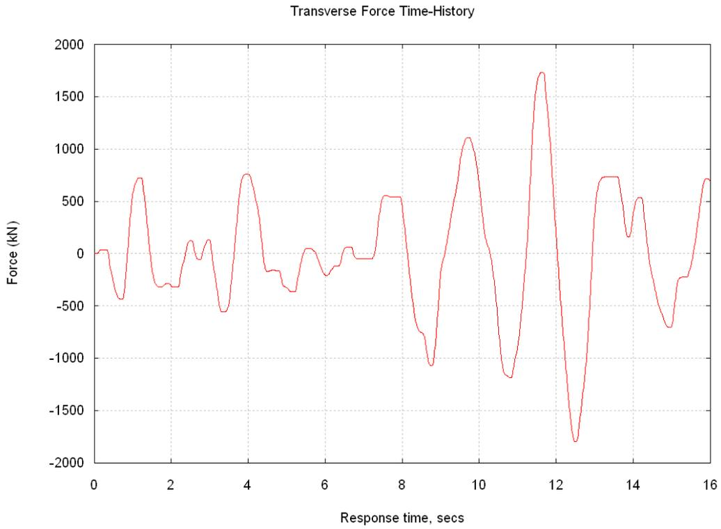
**Fig. 11– Typical transverse force time-history plot for selected pier**
