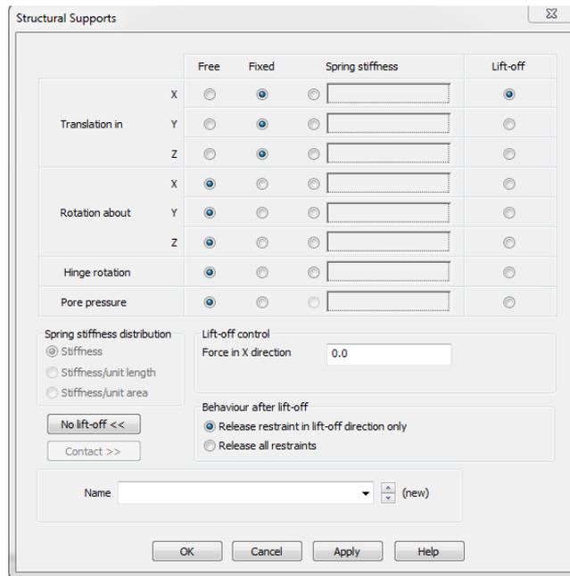
**Fig 1 – Lift-off control**
