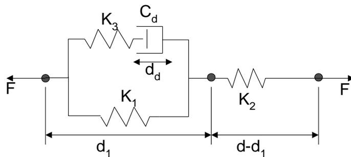
**Fig. 5– Four parameter solid model for visco-elastic bearings**
