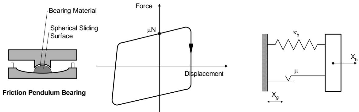
Friction pendulum bearing, hysteretic behavior and schematic representation
