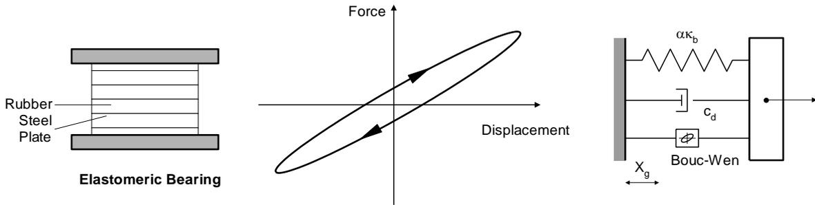
High damping rubber bearing, hysteretic behavior and schematic representation
