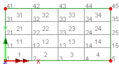
After: All nodes and elements renumbered using global directions.
