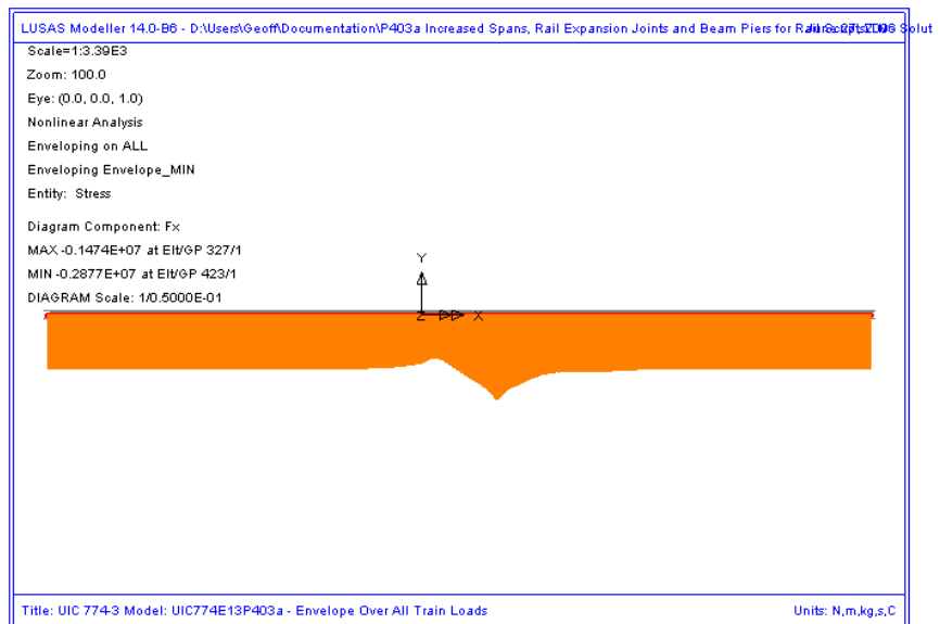
Figure 104: Axial Force In Rails Due To Combined Temperature And Enveloped Rail Loading
