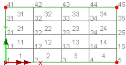
After: All nodes and elements renumbered using global directions.
