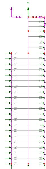
The Trilinear earth pressure material generates forces in the joint elements appropriate to the position (depth) of the joint element in the model. These forces must be resisted by supporting the free end of the joint elements.
