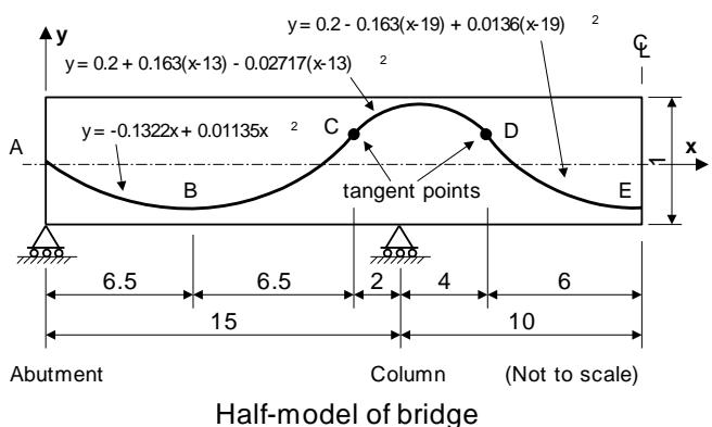
The initial post tensioning force of 5000 kN is to be applied from both ends. Tendons with a cross section area of  $3.5e3\text{mm}^2$  are located every 2 metres across the section allowing the analysis to model a 2 metres effective width.
