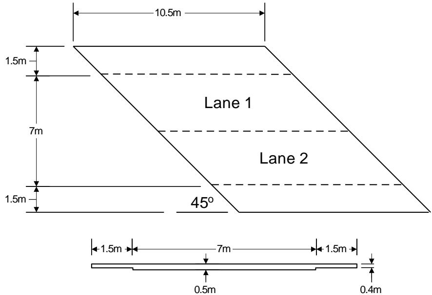
The structure is subjected to loading defined in the Departmental Standard BD 37/88 Loads for Highway Bridges.
