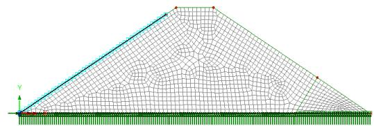
Select the lower inclined line of the upstream slope of the dam (Line 1 in the model) and from the
