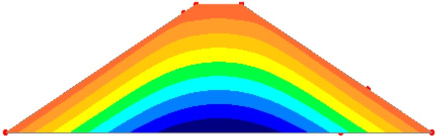
In the Displacement Reset Step loadcase, the deformations are set to zero (to match the as-built geometry) with in-situ stresses maintained
