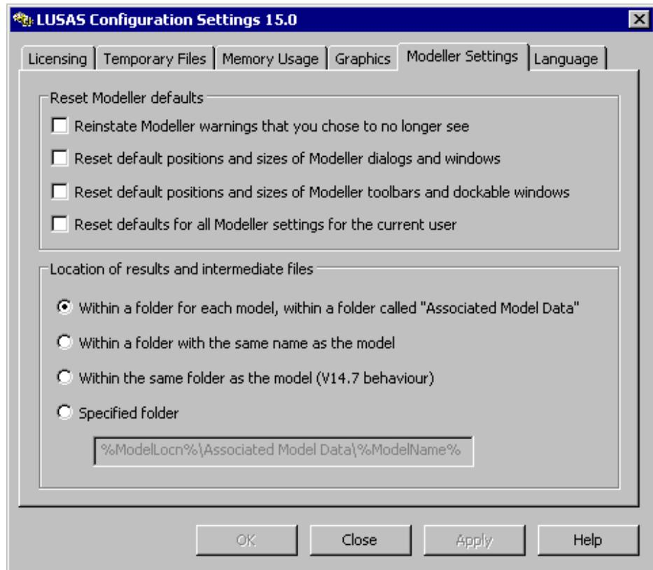
This page of the **LUSAS Configuration Utility** allows you to reinstate any Modeller warnings that you previously chose to stop the display of, reset the stated default Modeller settings for the current user, and control where LUSAS results and intermediate files are written to.
