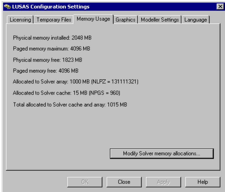
This page of the **LUSAS configuration utility** shows the physical memory (RAM) installed in your computer, and also how much of it is in use.
