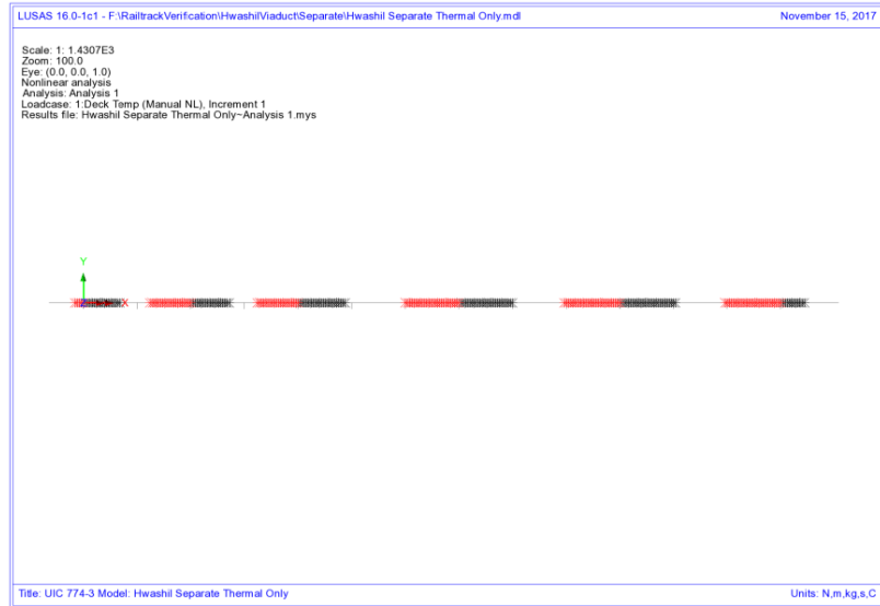
Figure 92: Track/Rail 1 Yield Due To Thermal Load On Track Alone
