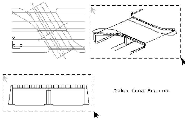
The DXF features are imported in scaled units defined by the drawing scale. These features will need to be scaled to suit the units of the analysis. Only the features
