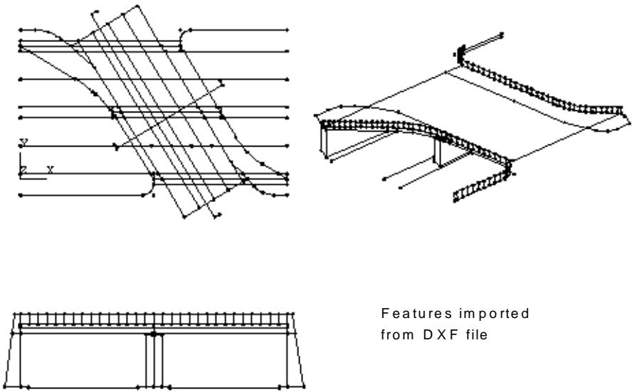
The initial geometry shown is equivalent to that imported from a typical CAD general arrangement drawing.
