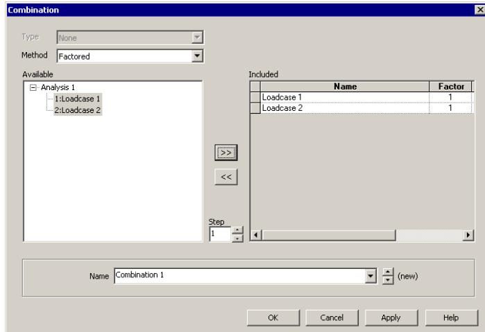
Both available results loadcases should be added to the Included combination panel.
