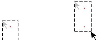
2. Drag a box around these two Points to create a vertical line on the centre line of the Frame
