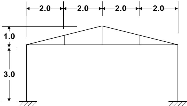
The structure is subjected to two loadcases; the self-weight of the structure, and a sway load at the top of the left-hand column.
