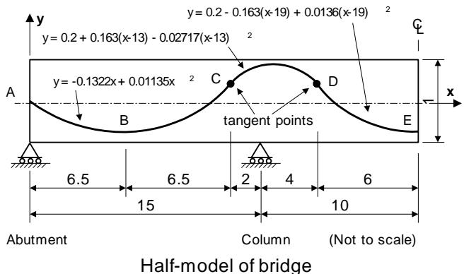
The initial post tensioning force of 5000 kN is to be applied from both ends. Tendons with a cross section area of  $3.5e3\text{mm}^2$  are located every 2 metres across the section allowing the analysis to model a 2 metres effective width.
