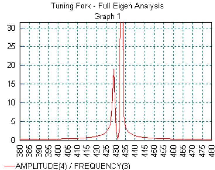
This displays a better representation of the displacement/ frequency response in the vicinity of the first two mode shapes.
