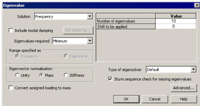
The following parameters need to be specified to perform a frequency analysis with a specified number of the minimum eigenvalues.
