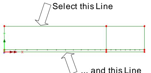
A graded mesh will be drawn on the left-hand Surface and a uniform mesh will be drawn on the right-hand Surface.
