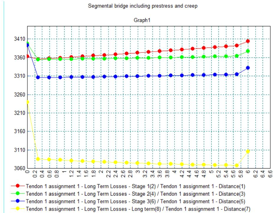
This shows the remaining prestress force (long term) in the tendon following each stage of construction.
