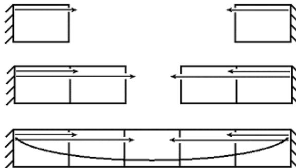
Each stage of the construction analysis considers a 6m long section being added to the construction. These are: Stage 1 (top-left), Stage 2 (top-right), Stage 3 and Stage 4 (middle) and Stage 5 (bottom).
