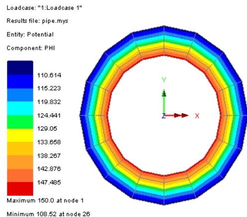
From the analysis it can be seen that the maximum temperature the outer surface of the pipe reaches is 108.5 °C.
