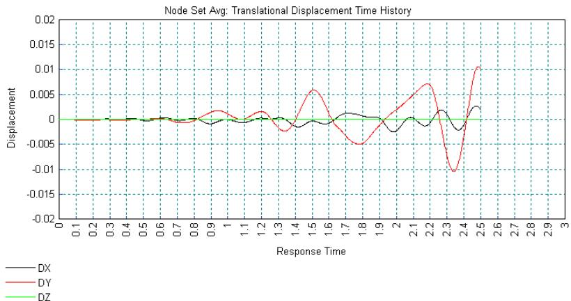
The peak results for the averaged node displacements are displayed in Notepad in file peak\_dspSet\_Avg1.sum. These indicate absolute peak average displacements of 0.0027m at time 2.4725 seconds in the X-direction and 0.0106m at time 2.485 seconds in the Y-direction.
