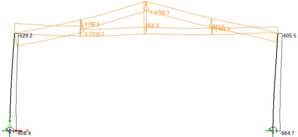
An axial force diagram for each member will be displayed with values of  $F_x$  displayed on the selected columns.
