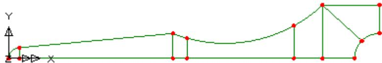
The remainder of the fork will be created by sweeping the vertical Line at the right-hand end of the model through a distance in the X direction.
