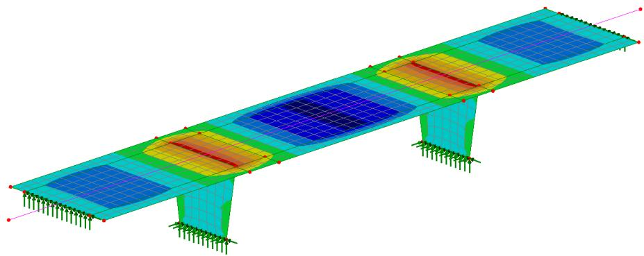
This shows the moments present in the deck and piers when no joints have been assigned to the model.
