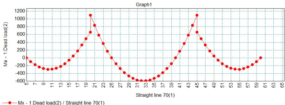
By hovering the cursor over graph points of interest it can be seen that the peak moment at the internal supports is 1092kNm and the lesser moment is 654kNm – meaning that the pier is currently attracting a moment of  $1092 - 654 = 438$ kNm.
