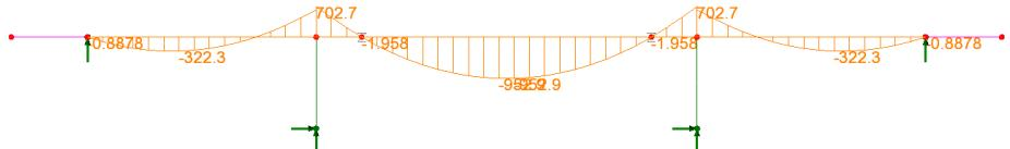
From the updated diagram it can be seen that the bending moment at the drop-in slab bearing location is effectively zero. There is a now a reduced amount of moment still in the piers which will be investigated next.
