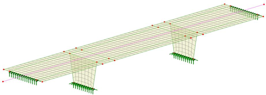
Groups have been defined for the features in the deck and the piers. These are used to restrict the extent of data used to create graphs of results along the deck. The line along the centre of the bridge is used when graphing results.
