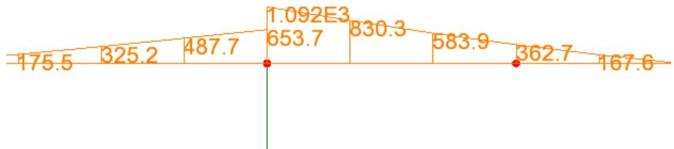
From the updated diagram the previously described bending moments at the support can be seen, and the moment at the intended drop-in slab bearing location is in the order of 363kNm.
