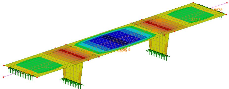
This shows that the bending moment at the location of the bearings (joints) of the drop-in span is zero as the joints don't have any rotational stiffness.
