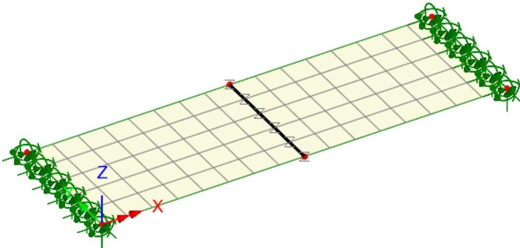
*Figure 4 – Joint mesh attribute assigned to line.*
