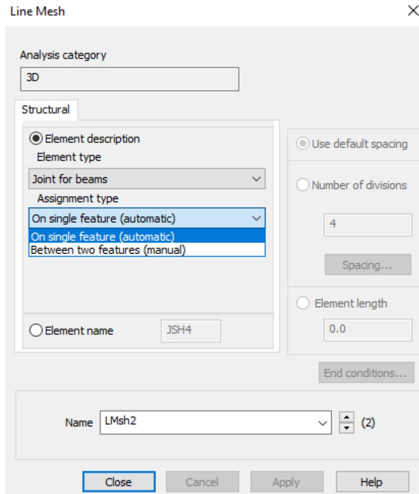
Figure 1 – Assignment type: On single feature (automatic).
