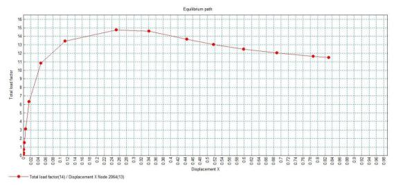
A decrease in the curve at total load factor 14.47 indicates a change of stiffness and it's the desired value i.e. the buckling load factor. The shape of the curve shows that after buckling the structures has an unstable behaviour i.e. there is a reduction in its stiffness.
