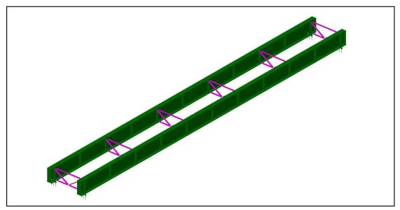
Thick quadrilateral shells with linear interpolation (QTS4) elements are used to mesh the plate girders and thick nonlinear beam (BTS3) elements to mesh the bracing trusses.
