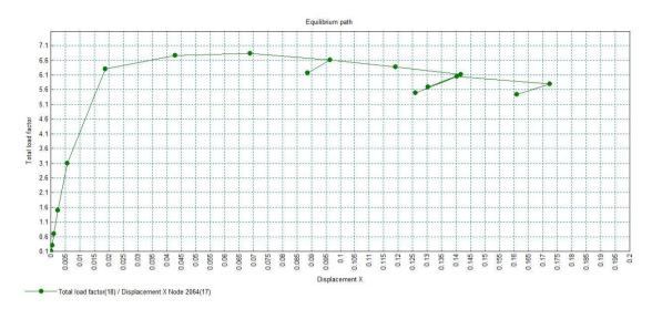
Note that there has been a few small unloading and re-loading increments due to use of Arclength method for achieving convergence.
