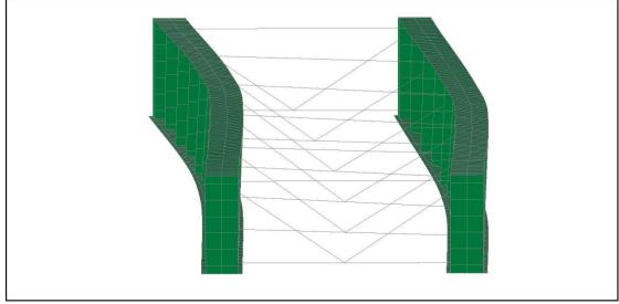
By using the alternative eigenvalue buckling solution the negative eigenvalues could be rectified, as this alternative algorithm will always give positive eigenvalues except when the buckling load factor is less than unity.
