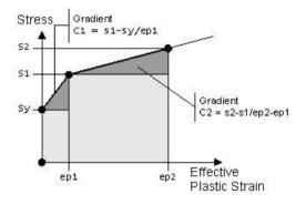
A small hardening slope is being used only for numerical reasons; a "zero" value could potentially lead to numerical instabilities and nonconvergence of the model.
