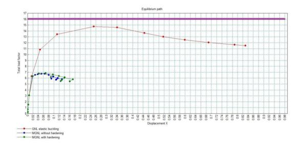
In the above graph all the curves from the different analyses are plotted together. The total buckling load factor from the eigenvalue analysis is the upper bound of the problem.
