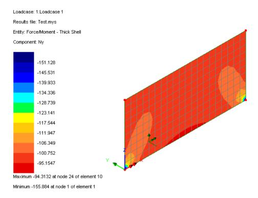
To maintain equilibrium this additional force is expected to result in a decrease in steel tensile force of 94.3/2 = 47.1 kN/m (to 82.2 kN/m) and an increase in concrete compressive force of 47.1 kN/m (to approximately 176.4 kN/m).
