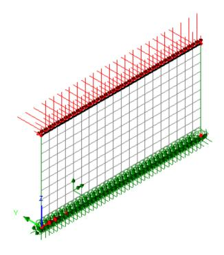
...the bending effects will not be changed but a compressive membrane force of approximately 100kN/m is introduced. The axial force value at the centre base of the wall is 94.3kN/m.
