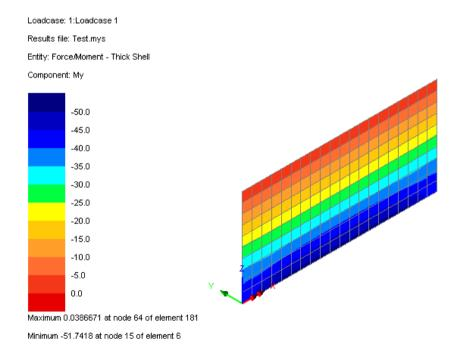
The vertical in-plane force is zero. Due to the direction of the loading and the orientation of the surface axes, tensile forces are expected in the bottom face y-direction reinforcement so Clark-Nielsen component **Ny(B)** is of interest. Orthogonal reinforcement is assumed and distance from top and bottom outer surfaces to centre of reinforcement are set to 50mm by pressing the 'Wood-Armer' button on the contour layer properties dialog.
