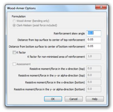
The Morley sandwich analogy assumes a lever arm of the section depth minus the top and bottom cover (i.e. 500 - 50 - 50 = 400mm = 0.4m in this case) therefore the expected maximum value of **Ny(B)** corresponding to the maximum moment of 51.74kNm/m is 51.74 / 0.4 = 129.35kN/m:
