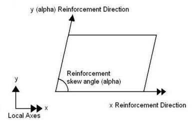
The "Reinforcement skew angle", also known as "alpha", is entered in the "Wood-Armer Options" dialog in LUSAS as shown in section 0 "
