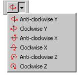
View along axis Views the model along a chosen global axis. Note that this toolbar button is not provided as part of the standard user interface but it can be added by selecting the View > Toolbars > Customise > menu item. This facility is also available by clicking in the X, Y or Z boxes in the Status Bar (holding-down the Shift key, if needed, to obtain the views along the negative screen axes.)
