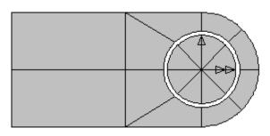
contact and the pin is then subjected to a prescribed concentrated loading and moved into contact with the lug.
