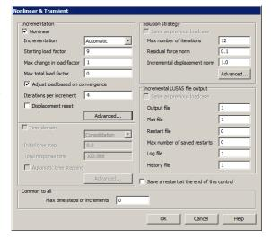
To terminate the load on a limiting variable the advanced nonlinear parameters need to be set in the Incrementation section.
