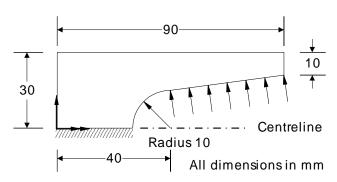
After an initial linear analysis with the specimen subjected to the pressure load, nonlinear material properties are defined and a nonlinear analysis is carried out using the same pressure loading.
