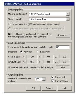
On the IMDPlus Moving Load Generation dialog set the Incremental distance to 0.1
