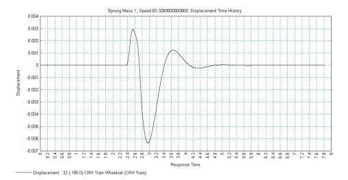
The graph shows that the sprung mass representing the body of the last wheelset of the train displaces almost 6.5 mm from its static position while it is over the continuous beam before the damping of the spring-mass system quickly damps out the body motion after the wheelset leaves the structure.
