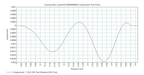
The second graph shows the curve after zooming into the first 0.5 seconds of the time history. This indicates that the displacement of the unsprung mass returns to zero (i.e. the first spring-mass system has left the structure) after about 0.48 seconds. This can be confirmed by dividing the total length of the continuous beam by the speed, 40 / 83.328 = 0.48 seconds.
