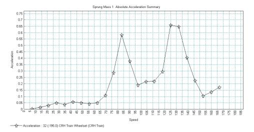
The graphs of the absolute peak vertical acceleration of the sprung bodies over the speed range appear to indicate that the peak acceleration increases as the number of wheelset spring-mass systems which have already passed along the beam increases. This is roughly true but from inspection of each wheelset spring-mass system it can be seen that the absolute peak acceleration out of the whole 32 wheelsets of the train actually occurs at the 30<sup>th</sup> wheelset, indicated in the graph below.
