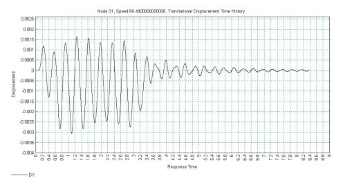
The graph generated shows the vertical displacement response at the mid-span of the second span of the continuous beam for the passage of the CRH trainset at 250 kph. The peak downwards deflection of the beam is approximately 3 mm and the peak upwards deflection approximately 1.6 mm. The response again matches the response of the second span in the Wang *et al* paper, noting that the sign conventions are opposite to the paper which has a positive vertical displacement in the downwards direction.
