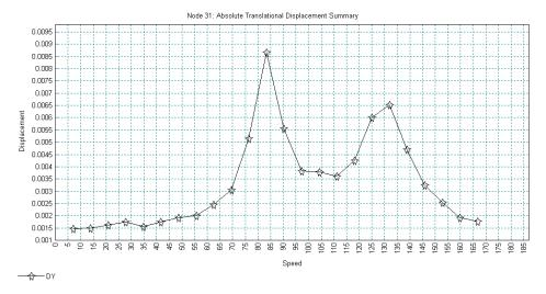
The graph shows that the worst vertical displacement response of the second span occurs again around 83.328 m/s which is equivalent to a train speed of 300 kph. At this speed the peak vertical displacement response is approximately 8.7 mm. A second peak is again observed between speeds of 124.992 m/s (450 kph) and 131.936 m/s (475 kph). Both of these peaks agree with the Wang *et al* paper and a more refined speed range would provide the same smooth curves in the paper.
