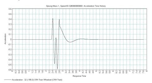
The graph shows the vertical acceleration response of the body of the last wheelset and indicates that it experiences a maximum acceleration of -0.582 m/s<sup>2</sup> or -0.059 g while it is about to leave the continuous beam. This peak acceleration for the last wheelset is significantly higher than the first wheelset as might be expected for subsequent
