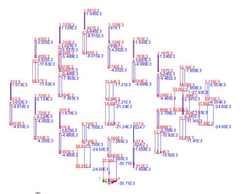
• In the  $\bigcirc$  Treeview right-click on the Whole Earthquake (Max) envelope and select the Set Active option to set this envelope active. Select entity Force/Moment of component My. Ensure that Change existing drawing layers to above component is selected, then click the OK button.
