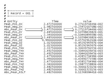
An envelope of the peak results for the chosen nodes is displayed in Notepad in file peak\_dspSet1.sum and is shown in the following figure. The peak X-displacement of 0.0068m occurs at node 143 at time 2.745 seconds and the peak Y-displacement of 0.0248m occurs at node 135 at time 2.49 seconds.
