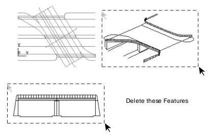
The DXF features are imported in scaled units defined by the drawing scale. These features will need to be scaled to suit the units of the analysis. Only the features
