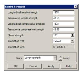
Click **OK** to update the contour key details and **OK** again to display contours of the Tsai Wu failure criteria.
