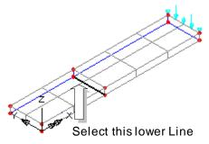
Surfaces that are, in effect, axes of symmetry for the entire strip. These supports are easier to assign on a view along the global Z axis.
