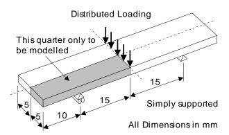
A 50mm x 10mm x 1mm thick composite strip, composed of an 8-layer composite material is to be analysed first using shell elements and then using solid elements in order to compare the results obtained.
