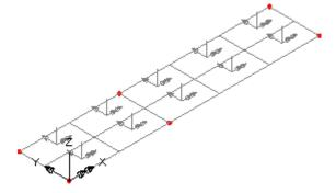
• Click **Apply** to rotate the axis by 90 degrees each time, until the x axis match with those of the left-hand surface.
