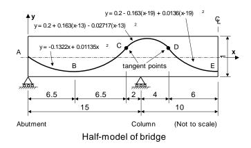
The initial post tensioning force of 5000 kN is to be applied from both ends. Tendons with a cross section area of  $3.5e3mm^2$  are located every 2 metres across the section allowing the analysis to model a 2 metres effective width.
