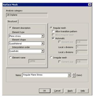
The mesh will be assigned to the model at a later stage.
