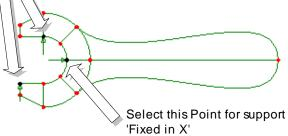
• Click the **OK** button to assign the support to the Point selected for all the loadcases in analysis 1.
