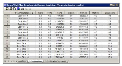
All beam/shell slice components are displayed in the Print Results Wizard Table. The axes defining the forces and moments are those displayed by the local coordinate system of each slice.
