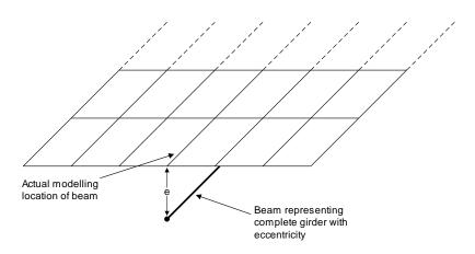
Beam element modelling of the whole girder
