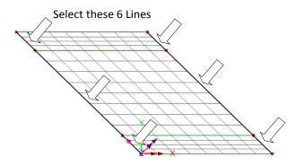
• Drag and drop the support attribute **Fixed in YZ** onto the selected Lines.
