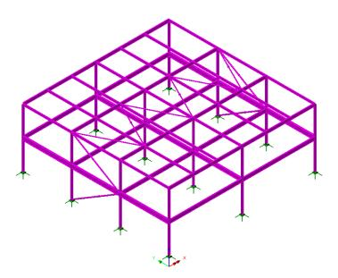
The frame consists of hot rolled structural steel sections, steel grade S 275, hot finished hollow sections, steel grade S 355 H and user-defined grade hollow section.
