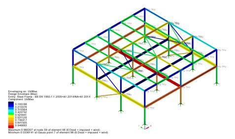
So it can be seen that, for this example, the illustrative results obtained by assigning revised section properties to a previously solved model very closely match the actual results obtained from re-solving the model using those revised properties.
