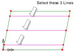
Additional Points will be created at mid-span and existing Lines will be broken into 2 new Lines. The new Points will be used later to define the position of the mid-span knife edge loads for each traffic lane.
