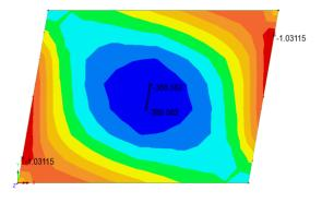
moment MY(B) equals the capacity of the slab MY\*(B). This would result in a restriction in the load carrying capacity of the slab.
