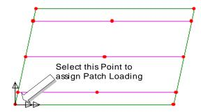
• Enter the loadcase as Lane load (lower) with a load factor of 1 and click OK
