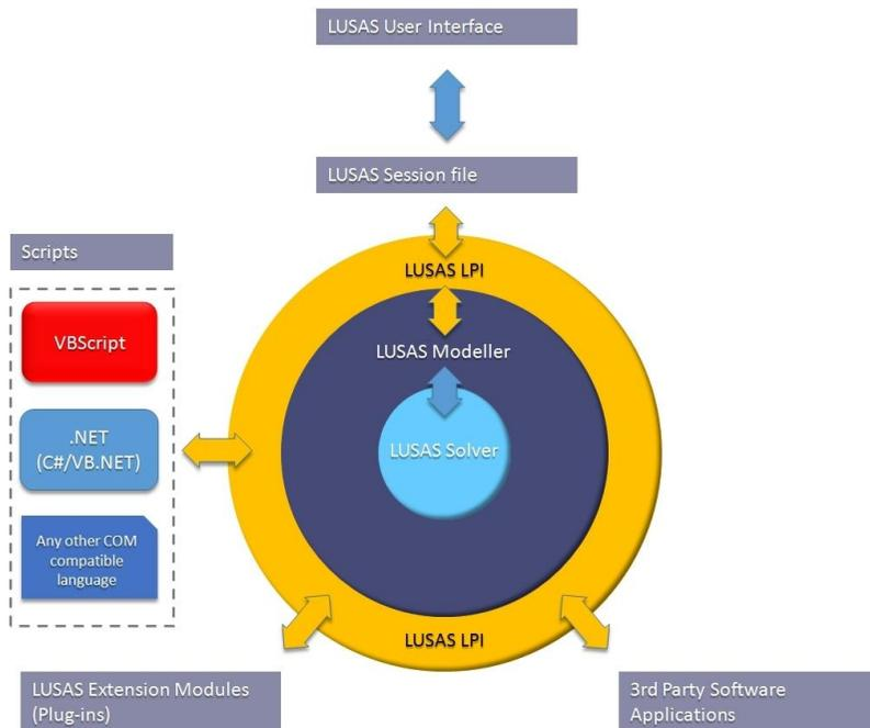
With LPI, any user can automate the creation of complete structures, either in LUSAS or from third-party software, carrying out design checks, optimising members and outputting graphs, spreadsheets of results and custom reports. Because everything carried out by a user is recorded in a LUSAS Modeller session file, anything that LUSAS can do, can also be controlled by another application via the LUSAS Programmable Interface. This means that you can view and edit a recorded session,
