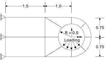
modulus of 210E9 N/m<sup>2</sup>, a Poisson's ratio of 0.3 and a mass density of 7800kg/m<sup>3</sup>.
