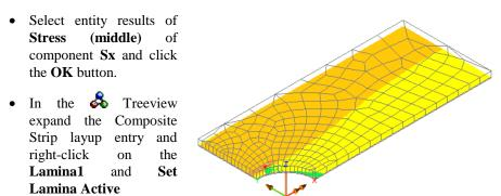
The contour key should be showing a maximum stress in the lamina X material direction of around 1.8E3
