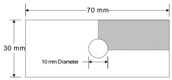
by a 10mm diameter hole. Because of symmetry a quarter model will be created.
