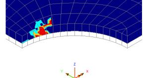
• By changing the active loadcase it can be seen that no failure has occurred after the first load increment (a load factor of 0.5). By the second load increment (a load factor of 0.75) a small amount of matrix failure has occurred adjacent to the hole.
