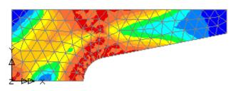
area shows the peak von Mises stress which is being limited to 300 N/mm<sup>2</sup> by the zero hardening slope as defined in the plastic material properties section for the model.
