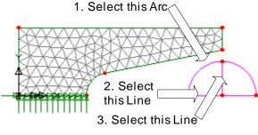
Geometry Surface By Lines... The right-hand Surface of the bolt will be drawn.
