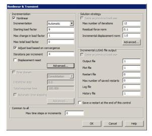
To terminate the load on a limiting variable the advanced nonlinear parameters need to be set in the Incrementation section.
